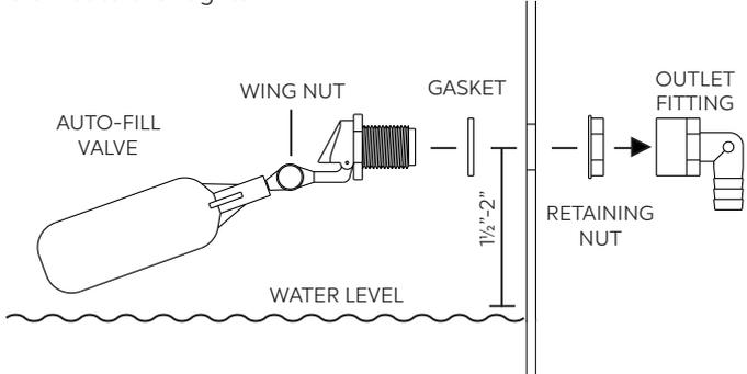
The Auto Fill Kit includes fittings for connection to a garden hose, ½" irrigation line, and ½" Sch 40 PVC. Wrap the ½" male threads on the Auto Fill with thread sealant and install the fitting of your choice. Once water is supplied to the Auto Fill it will maintain the set water level by automatically adding water when the level drops. This level can be adjusted by loosening the wing nut and raising and lowering the height of the Auto Fill float.
