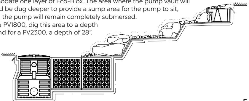
For installations where a larger basin volume or deeper basin is required, Atlantic offers pump vault extensions for both the PV1800 and PV2300. Each extension will add the height of one Eco-Blox. For each additional Eco-Blox layer, increase the depth of your excavation by 17".
