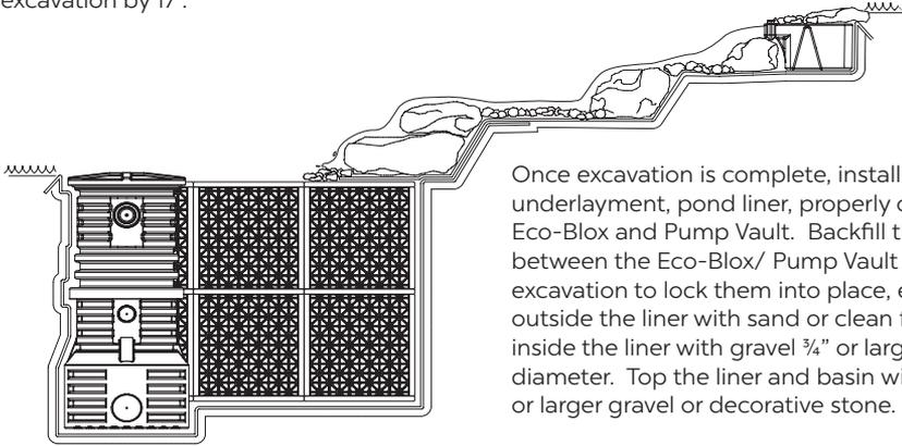
Once excavation is complete, install underlayment, pond liner, properly oriented Eco-Blox and Pump Vault. Backfill the space between the Eco-Blox/ Pump Vault and the excavation to lock them into place, either outside the liner with sand or clean fill, or inside the liner with gravel  $\frac{3}{4}$ " or larger in diameter. Top the liner and basin with  $\frac{3}{4}$ " or larger gravel or decorative stone.
