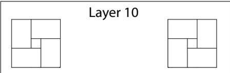
Finish the columns to the height desired (Layer 10). Cap the spillways with the final course of stone.
