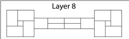
The next levels will accept the spillway option chosen. Colorfalls and Color Changing Colorfalls will need notches prepared to accept the base of the Colorfalls and the lip. Stainless Steel and Copper Finish Spillways replace 4-inch high block; leave out one 12-inch block for the 12-inch Spillway, 2 for the 24-inch Spillway, etc (Layers 7-9). Refer to spillway instructions for details.
