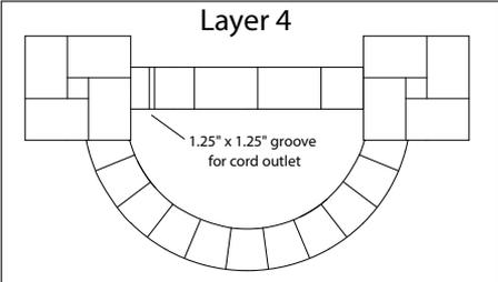
Continue setting stones until the walls of the basin have been completely covered (Layers 2-3). Leave a 1 1/4" x 1 1/4" hole for the the pump cord and thread the cord through. (Layer 4).
