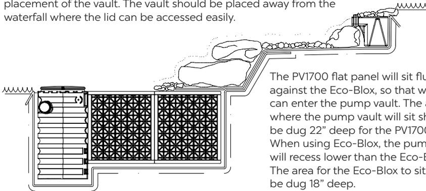
The PV1700 flat panel will sit flush against the Eco-Blox, so that water can enter the pump vault. The area where the pump vault will sit should be dug 22" deep for the PV1700. When using Eco-Blox, the pump vault will recess lower than the Eco-Blox. The area for the Eco-Blox to sit should be dug 18" deep.
