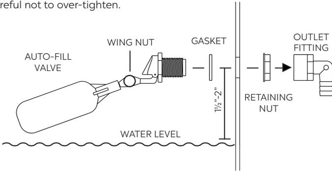
The Auto Fill Kit includes fittings for connection to a garden hose, ½" irrigation line, and ½" Sch 40 PVC. Wrap the ½" male threads on the Auto Fill with thread sealant and install the fitting of your choice. Once water is supplied to the Auto Fill it will maintain the set water level by automatically adding water when the level drops. This level can be adjusted by loosening the wing nut and raising and lowering the height of the Auto Fill float.
