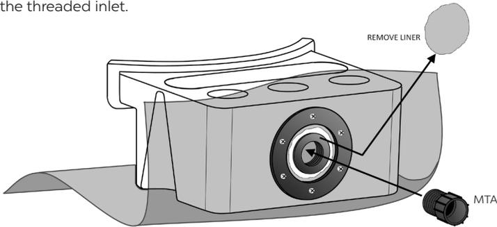
**Tighten flange screws with a hand held screwdriver only. Over tightening the screws could strip out the inserts or crack the liner flange. The screws need only to be snug for the silicone to make a seal.**
