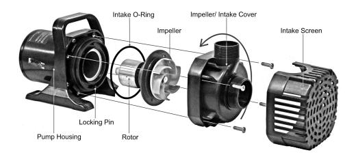
**NOTE:** If debris has accumulated around the rotor, the impeller may feel tight. Rotate the impeller back and forth while applying outward pressure until the impeller assembly wiggles free.
