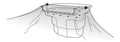
Remove the spring clips and pull the liner away from the face of the enclosure. Make sure that the front of the FilterFalls and the back side of the liner are clean and free of debris. Apply a full, continuous bead of Atlantic fish-safe RTV silicone to the face of the FilterFalls along the center line of the threaded inserts.
