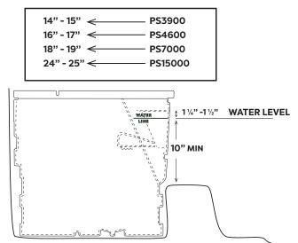
Place the Skimmer enclosure into the excavated hole. Check the top of the enclosure to make sure that it is level front-to-back and side-to-side. Check where your pre-determined water level falls on the face of the Skimmer enclosure. The water level needs to be between 11/4" and 11/2" below the top of the weir door opening and/or even with the water level indicator molded on the side of the Skimmer.
