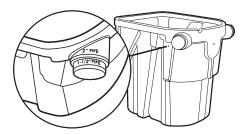
this water feature. Once completed, push one end of the PVC supply line through the step fitting allowing approximately 10" of pipe to enter the skimmer enclosure.
