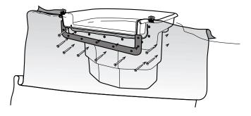
Attach the liner flange to the FilterFalls, starting with the center screw first, and then work out toward the sides of the spillway. It may be necessary to first pierce the liner with a nail or an awl before inserting the screw. Do not fully tighten any screws until all the screws have been installed. Once completed, trim away any excess liner as needed.
